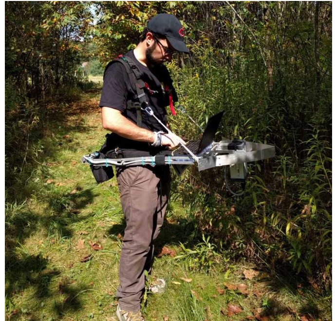
Figure 1. Portable Canopy Lidar (PCL) system being used to measure 2-D forest canopy structure. The PCL system is mobile and efficient for measuring canopy structure.
