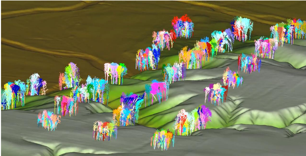
Figure 1. A Digital Terrain Model of a portion of Purdue’s Martell Forest populated by the individual trees extracted from terrestrial laser scans of each inventory plot. These digital plots allow algorithms to be developed for automatic feature extraction from point cloud data. The results of which can then be checked against the on-the-ground measurements collected by this project at each plot.
