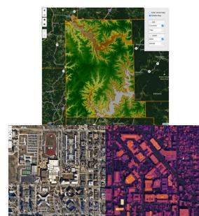
The Indiana LiDAR data portal project provides a public accessible visualization platform for several geospatial data products derived from the Indiana Statewide LiDAR data (top: DTM, bottom left: Aerial Imagery, bottom-right: NDHM).
